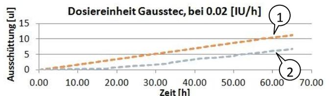
Fig 3: Long-term measurement with dosing unit Gausstec, without (1) and with interference (2)
